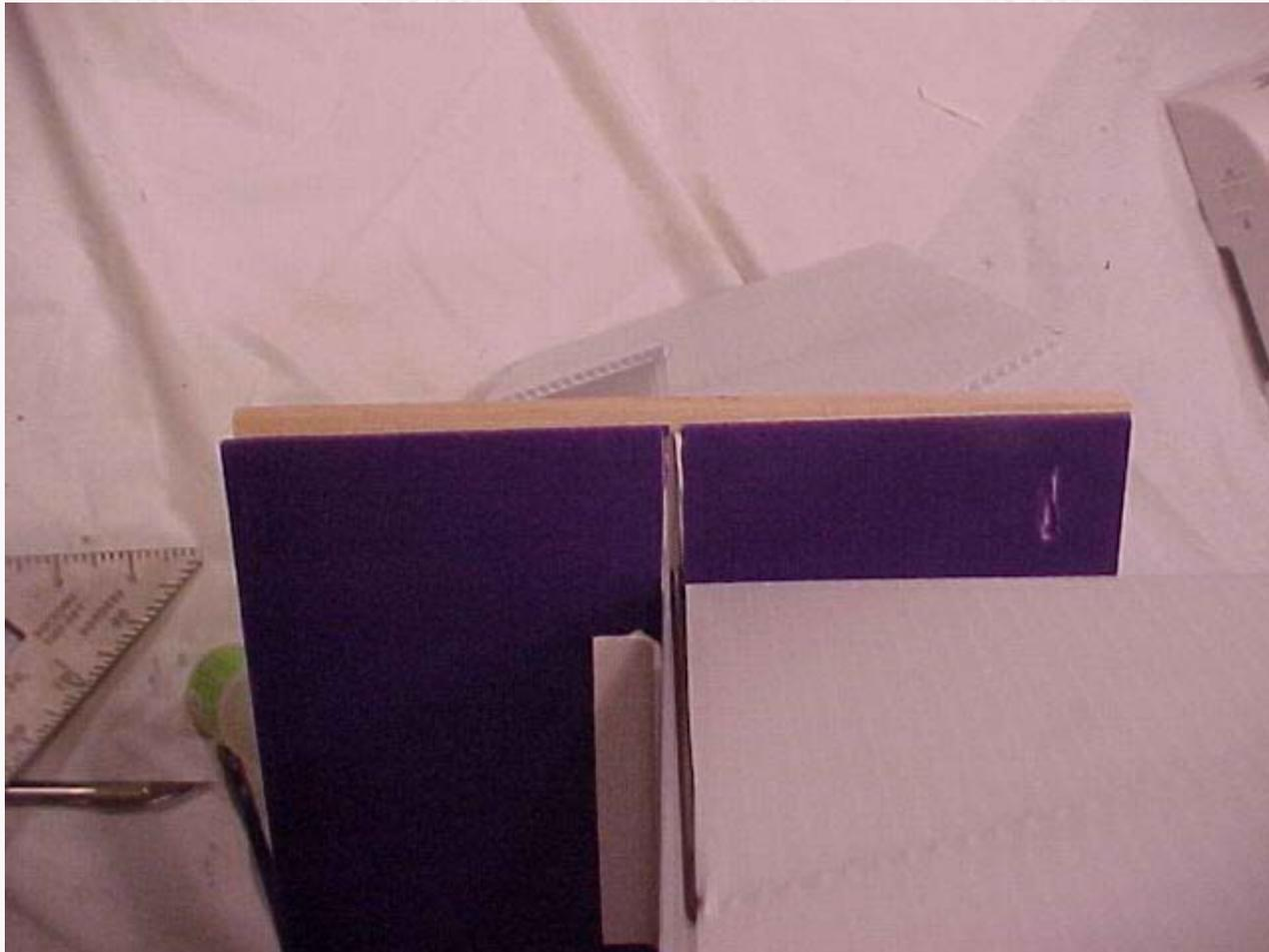
Next, align the rudder with the fuselage, and drill the dowel for the hinges.
