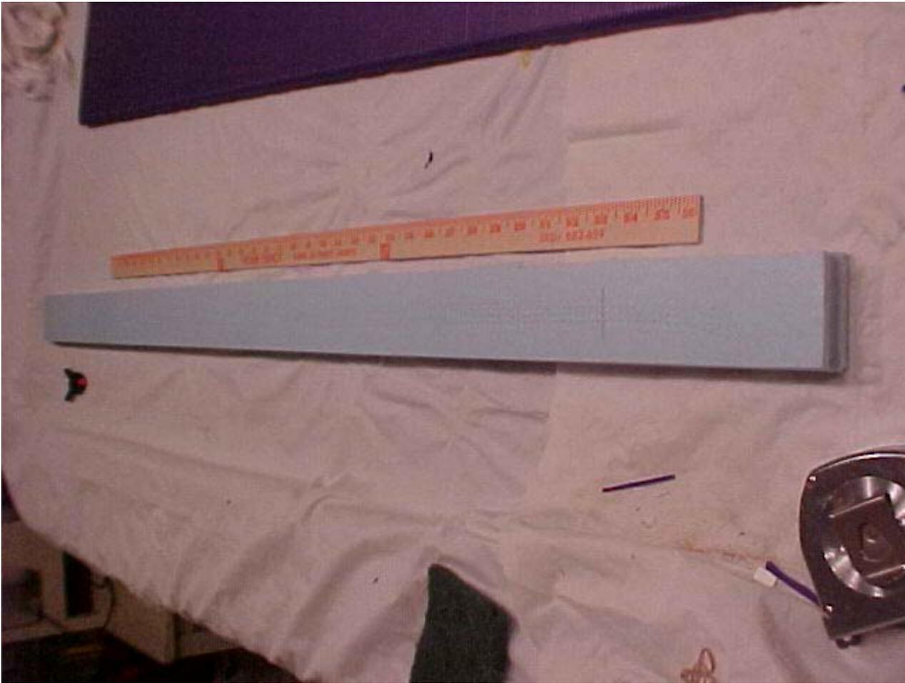
Next, wet the yardstick with water mist, and put a bead of polyglue down the center of the spar.
