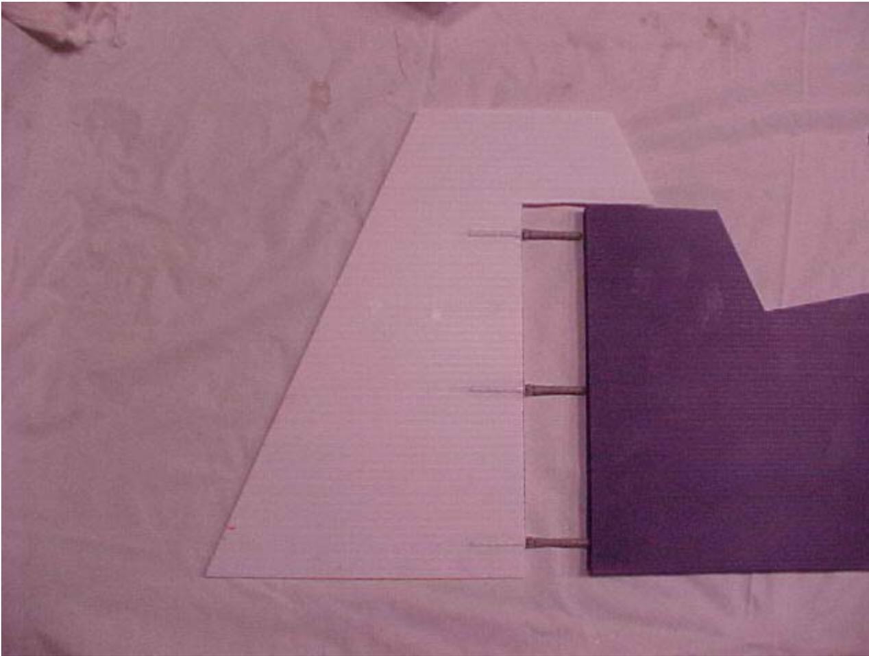
Locate the hor. stab dowel in the fuselage, and cut a slot out, from the trailing edge, forward 6" just above the dowel inside the fuse, and just wide enough for the hor. stab to slide in place.
