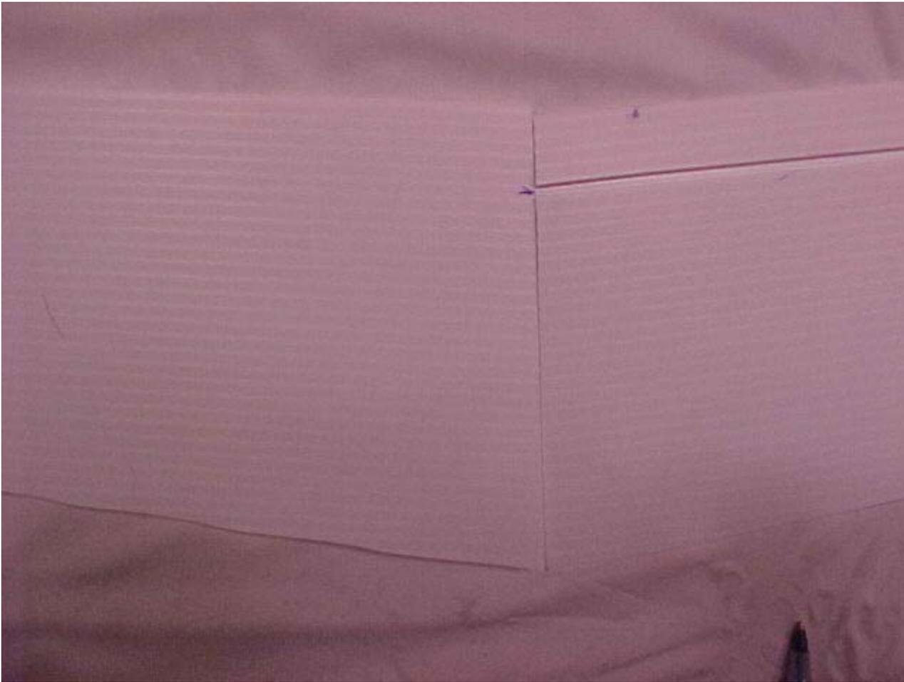
Now, mark the center of the wing. This is the center fold line. Mark a line  $\frac{3}{8}$ " on each side of the fold line. Score all 3 folds.
