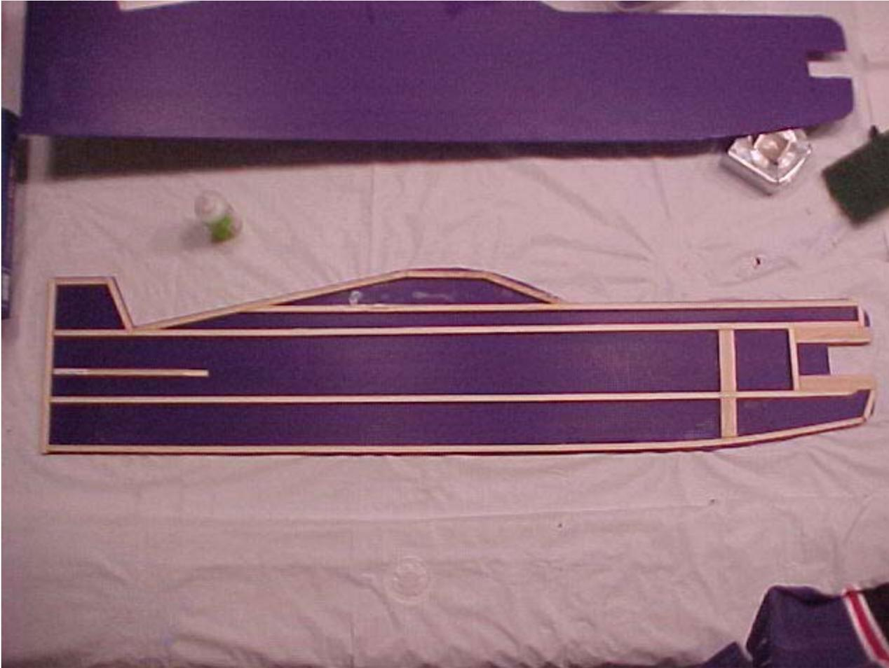
Put some books on top of the fuselage to hold it nice and flat until the glue dries. Preferably for a half hour or so. Here is the completed fuselage.
