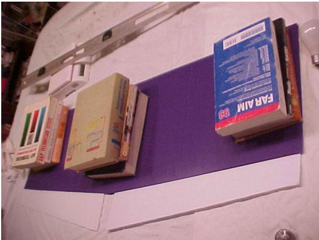
Once you get the wing skin aligned, and weighted as shown. Insert the tip of a ca bottle between the top wing skin, and the aileron (the portion inside the wing), and run a bead of ca down the aileron, to glue it in place. Very carefully pull the books up, one stack at a time, so they are weighting the top skin/aileron glue joint down. Being careful not to move the top wing panel.
