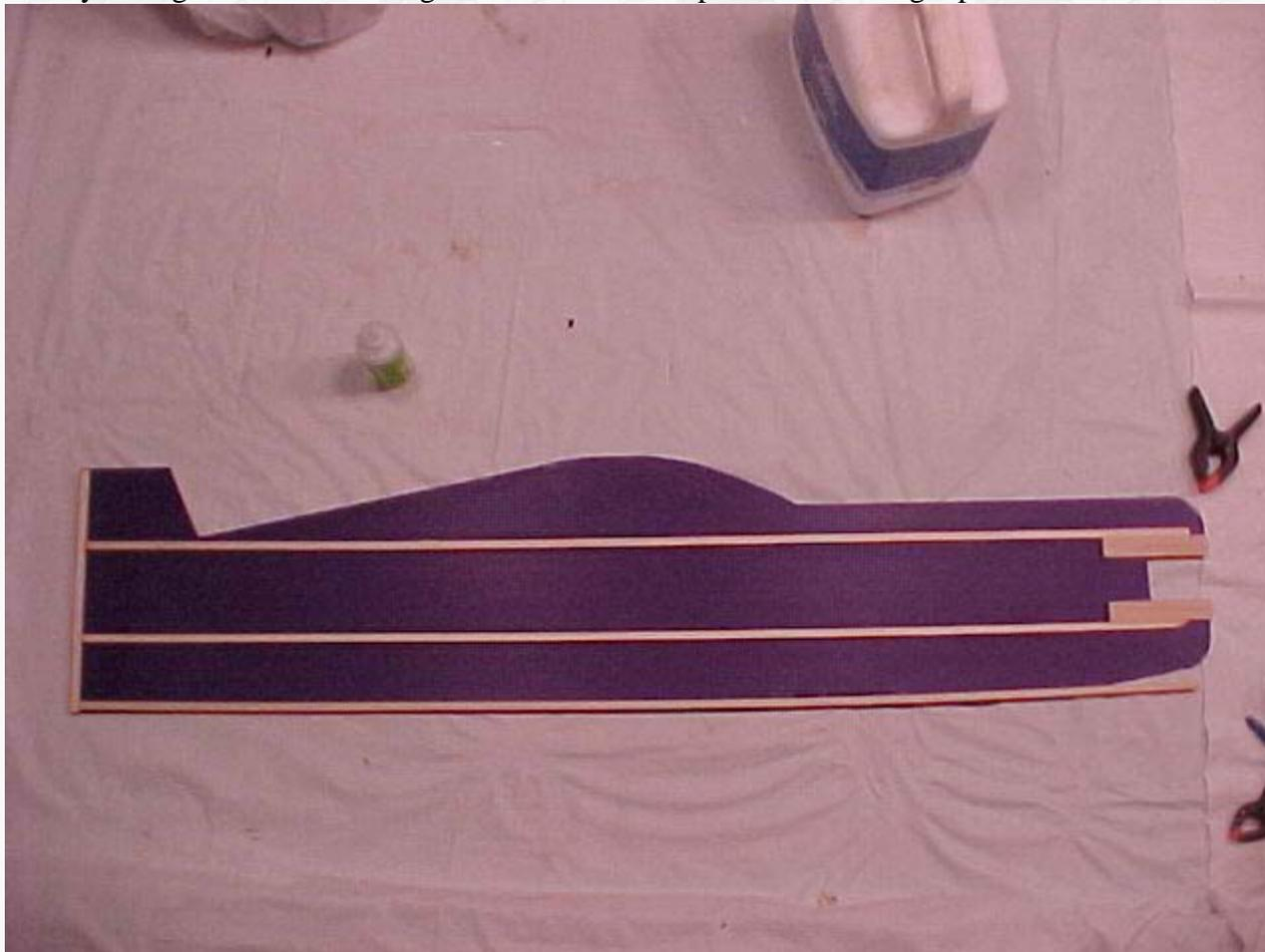
Let that portion dry. You can hit it with kicker if you'd like to speed up the process. Once dry, apply glue to the fuselage, and bend the stick up into position. Use plenty of ca, and then hit it with kicker to hold it in place. Then put some weight on it to be sure.
