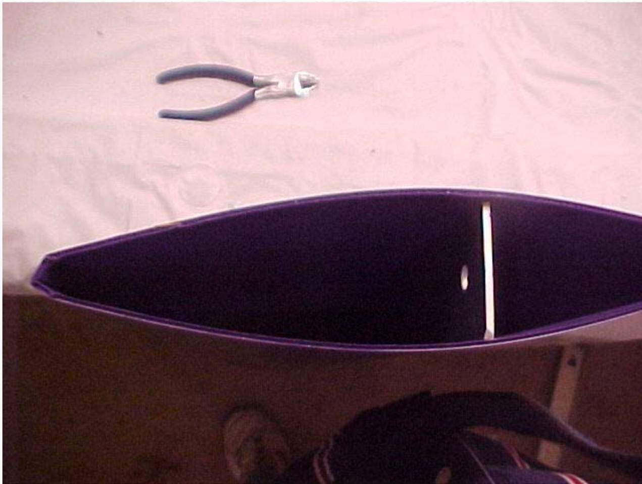
Wet the sides of the foam that polyglue to the coro with a water mist, and wipe off the excess. Then apply a generous bead of polyglue to the spar, both top and bottom.
