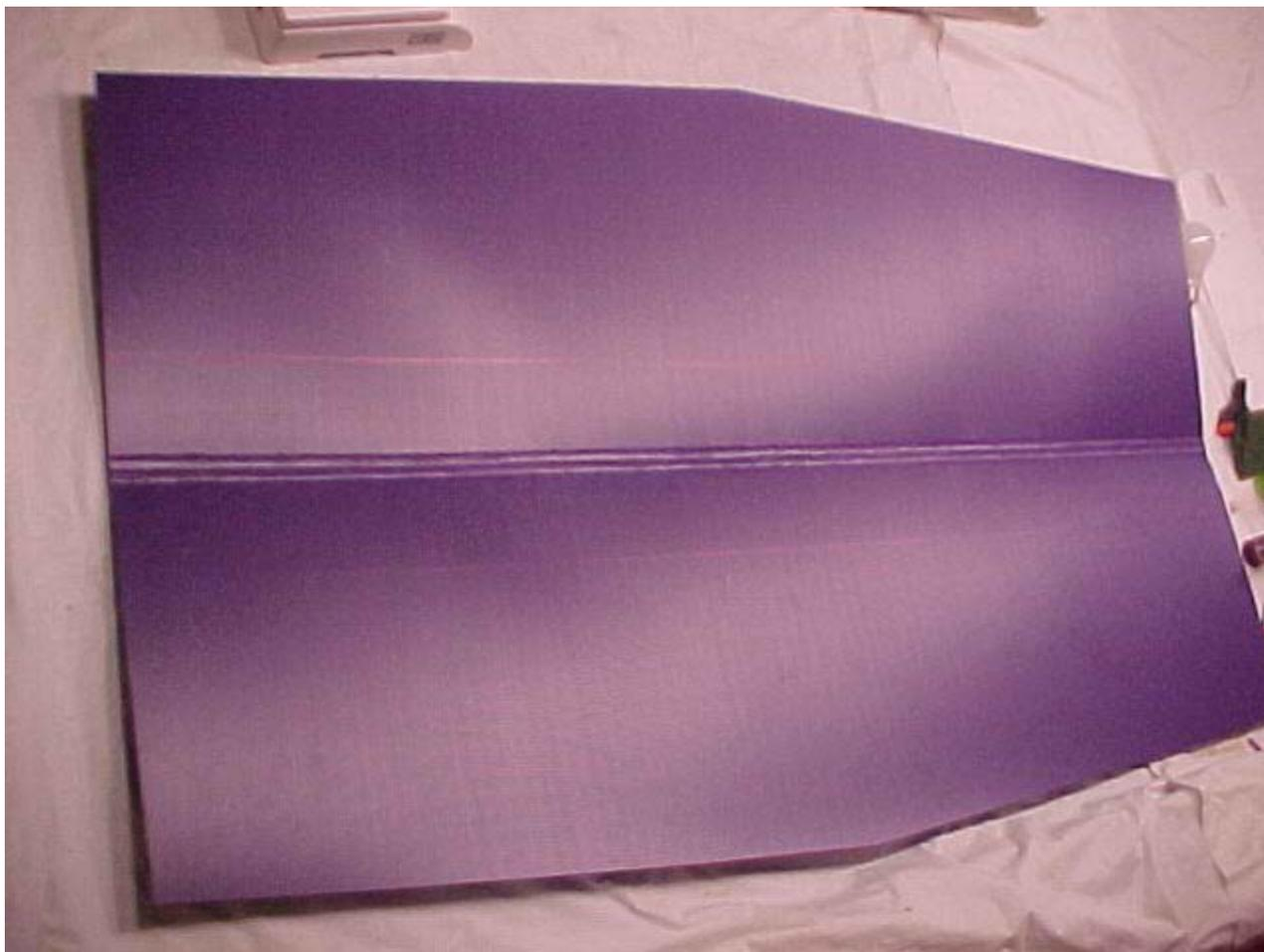
Now you need to prep the coroplast. Prep the entire inside of the wing, and the portion of the ailerons that will glue inside the wing using the mineral spirits and scotchbrite method described earlier, or whatever works for you.
