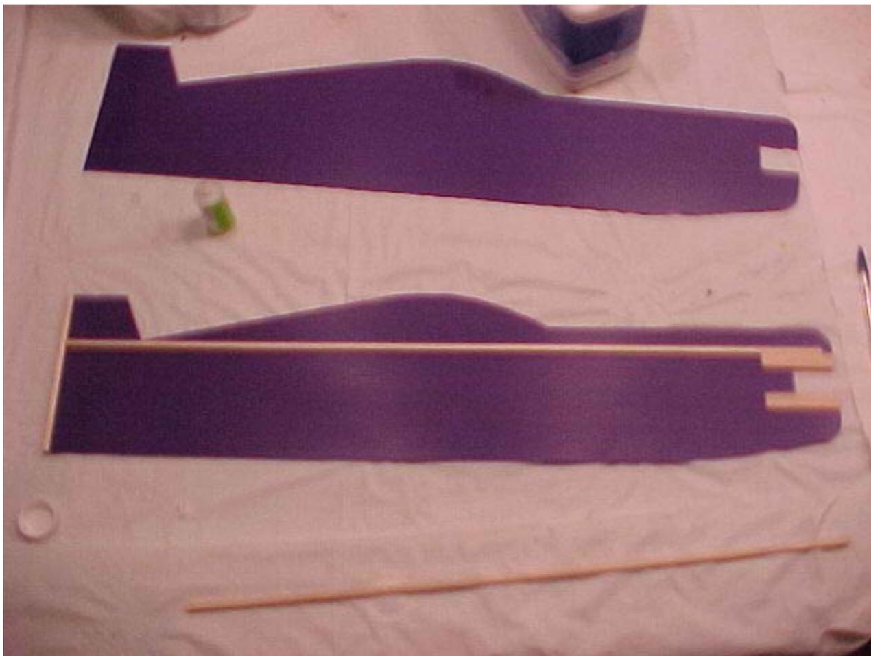
also mark the place where the dowel stops on the engine bearer. Glue the dowel to the bearer, and also do the same for the bottom rail and dowel. Then glue the top rail in place, and place some books on it to keep it nice and flat until the ca cures.
